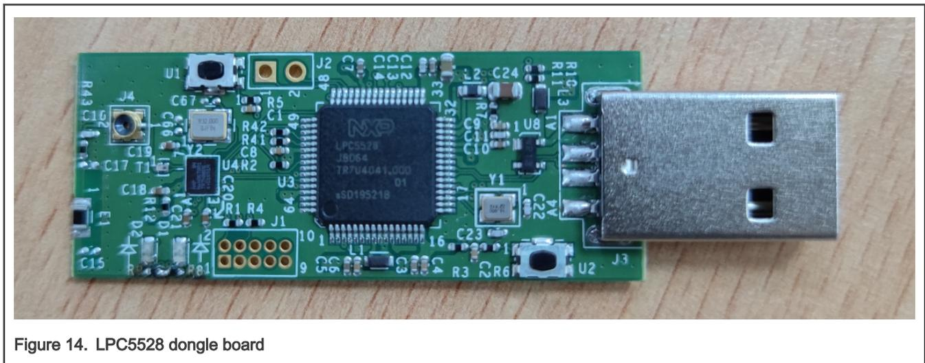
Figure 14. LPC5528 dongle board
