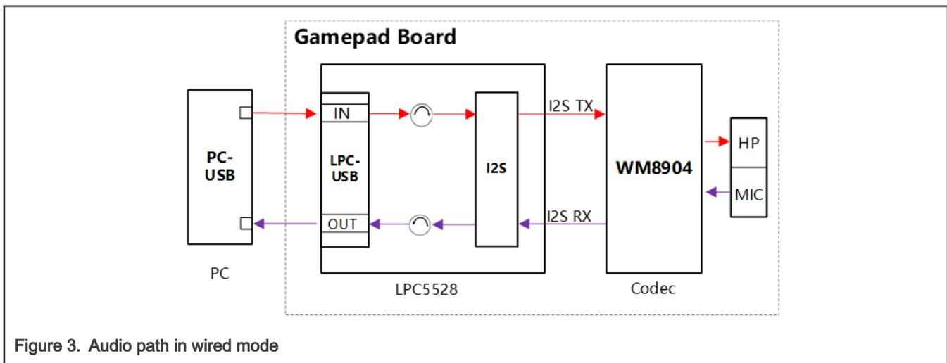
**Figure 3. Audio path in wired mode**
