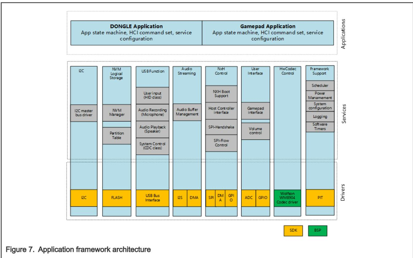
Figure 7. Application framework architecture
