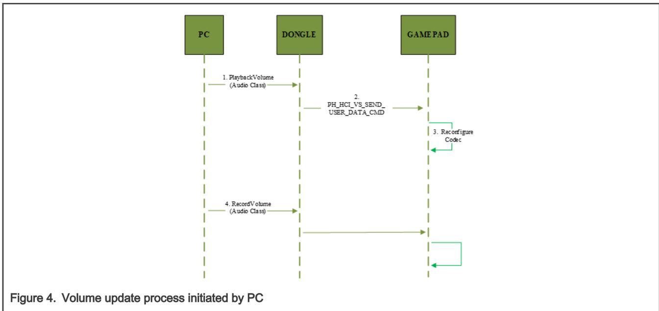
1. The user changes the volume setting on the PC. A USB volume update command is sent to the dongle.
