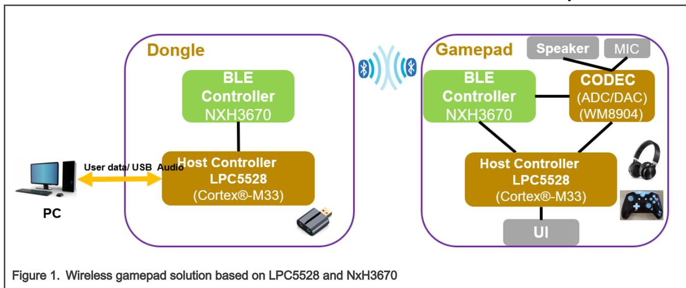
Figure 1. Wireless gamepad solution based on LPC5528 and NxH3670
