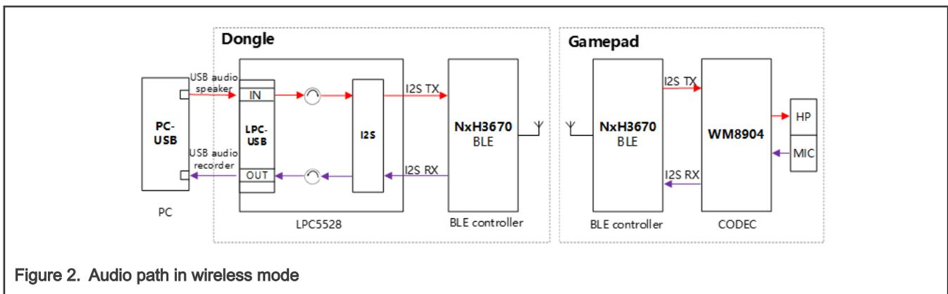
Figure 2. Audio path in wireless mode
