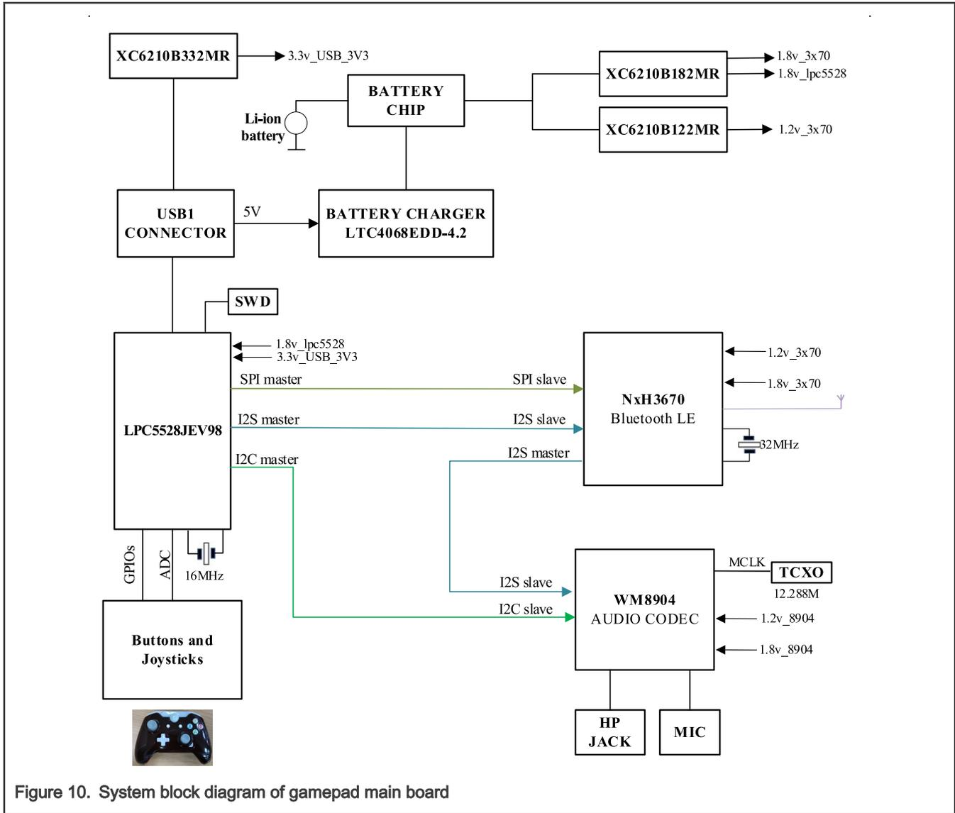
Figure 10. System block diagram of gamepad main board
