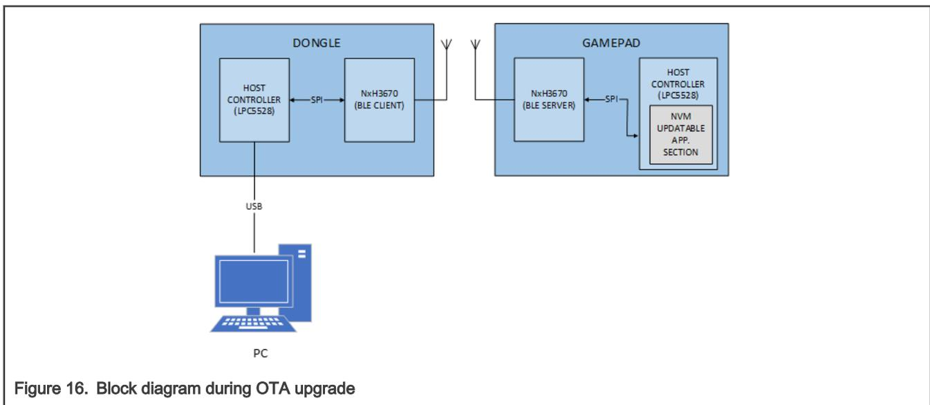
Figure 16. Block diagram during OTA upgrade
