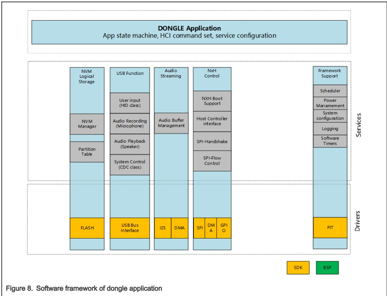
Figure 8. Software framework of dongle application
